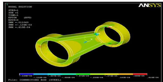
Fig: 7.9: Strain Analysis of Connecting Rod (Forged Steel)
