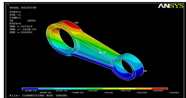
Fig: 7.2: Displacement of Connecting Rod (Magnesium Alloy)
